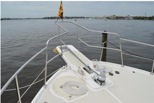
Bow Pulpit and Anchor Locker Hatch
